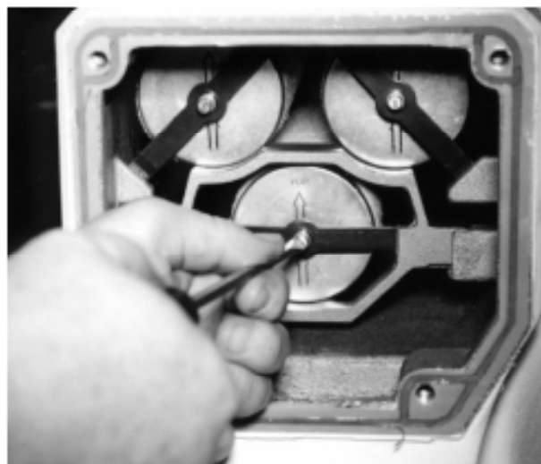
Fig. 3 - Removing Filter Spring
